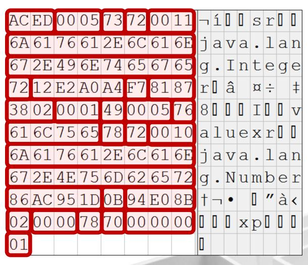
STREAM MAGIC STREAM VERSION OBJECT TC<sup>-</sup>CLASSDESC Class description length (17) Qualified class name Serial version UID **Description flags Object** handle Field count (1) Field type còde (int) Field name length (5) **Field name** TC ENDBLOCKDATA TC CLASSDESC Class description length (16) **Qualified class name** Serial version UID **Description flags Object handle** Field count (1) TC ENDBLÒCKDATA TC NULL The actual value (1)
